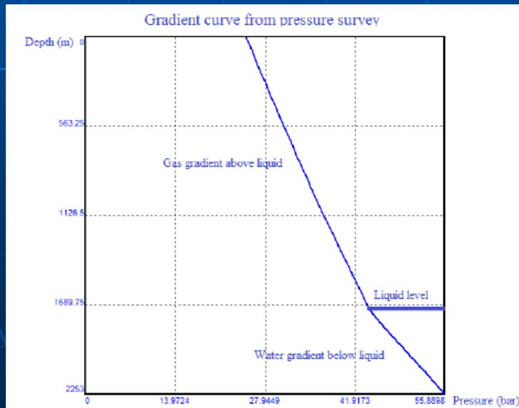
**Actual height of accumulated water** can be found from the gradient curve
