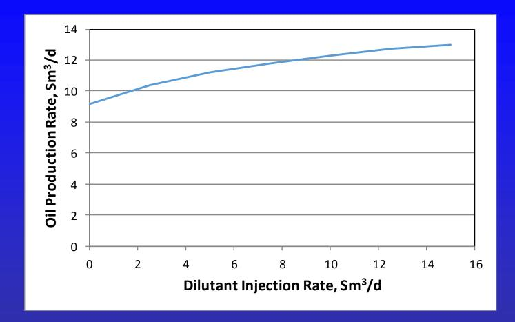
To Decrease Viscosity and Pour Point Constant Effect, Production Break Problems Eliminated Must be combined by artificial lift!
