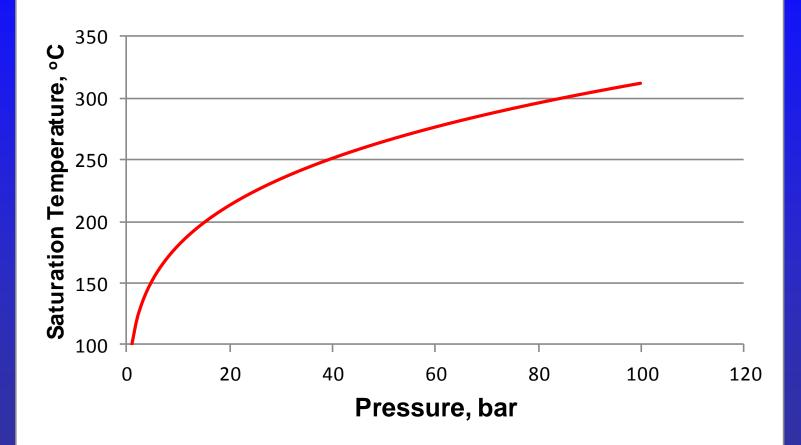
Required Minimal "gas lift pressure" - 30 bar ~ 220 °C Examined 305 °C ~ 80 bar
