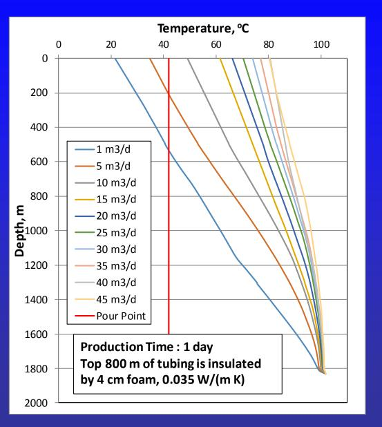
Reduced Deposition on Pipe Wall!
