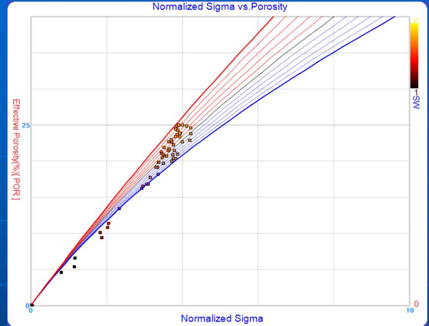
$$\Sigma_{\log} = \underbrace{V_{sh} \times \Sigma_{sh}}_{\text{SHALE}} + \underbrace{(1 - V_{sh} - \Phi) \times \Sigma_{ma}}_{\text{MATRIX}} + \underbrace{\Phi \times S_w \times \Sigma_w}_{\text{PORE SPACE}} + \underbrace{\Phi \times (1 - S_w) \times \Sigma_{hc}}_{\text{PORE SPACE}}$$
